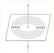
The direction of magnetic field lines can be found using the right-hand thumb rule. The magnetic field lines will be directed by the fingers wrapped around the current-carrying conductor if the conductor is held in the right hand with the thumb pointing in the direction of the current.
