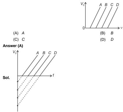
As per the variation shown above, for the same frequency of incident radiation the work function for metal *A* is minimum hence the kinetic energy of photo electrons will be maximum for metal *A*.
