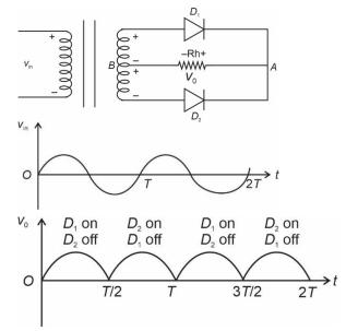
During positive cycle diode  $D_1$  is on and  $D_2$  is off. The current will flow through load resistance ( $R_L$ ) from A to B. For negative cycle diode  $D_2$  is on and  $D_1$  is off but direction of current through load resistance ( $R_L$ ) is still from A to B. The output is always in same direction irrespective direction of input.
